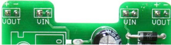
Solder those header pins on the top side of the PCB.
