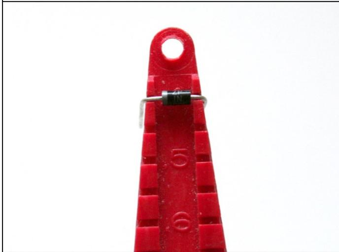
Use lead forming tool and bend diode's leads marked "**1N4005**" using .4 spacing. The lead forming tool can be purchase on our website P/N TOOL-BEND. You can also use needle-nose pliers to bend the leads.
