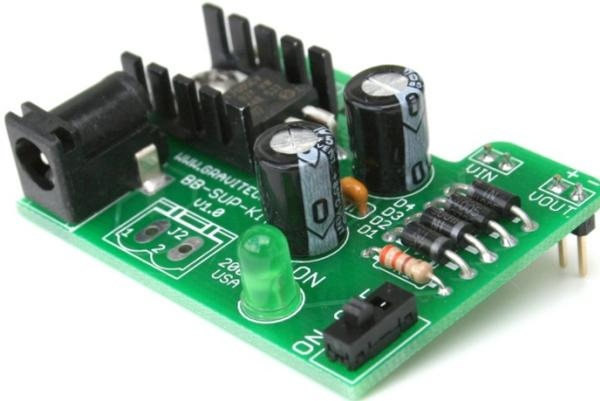
If you are using bench power supply, 9V battery or battery pack considers using 2 positions terminal block. It can be purchase separately P/N TERM-BLK-2. This terminal block can be place on J2 and now you have a quick way to connect and disconnect the power.
