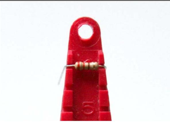
Use lead forming tool or needle-nose pliers and bend 330 Ohm resistor's leads using .4 spacing.
