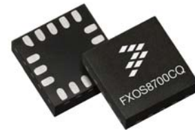
16 LEAD QFN 3 mm x 3 mm x 1.2 mm
